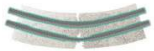
Steel design = Rebar Ductile Failure
