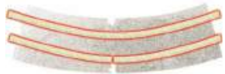
FRP design = Balance Brittle Failure
